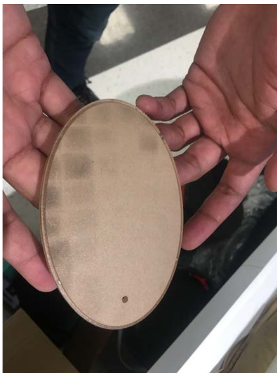
Figure 47: The surface of the acrylic is shiny and tacky after the repositionable adhesive spray.
