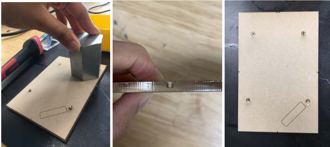
Figure 26: Insulated weight applied to the heat-set for flush insertion into pocket
