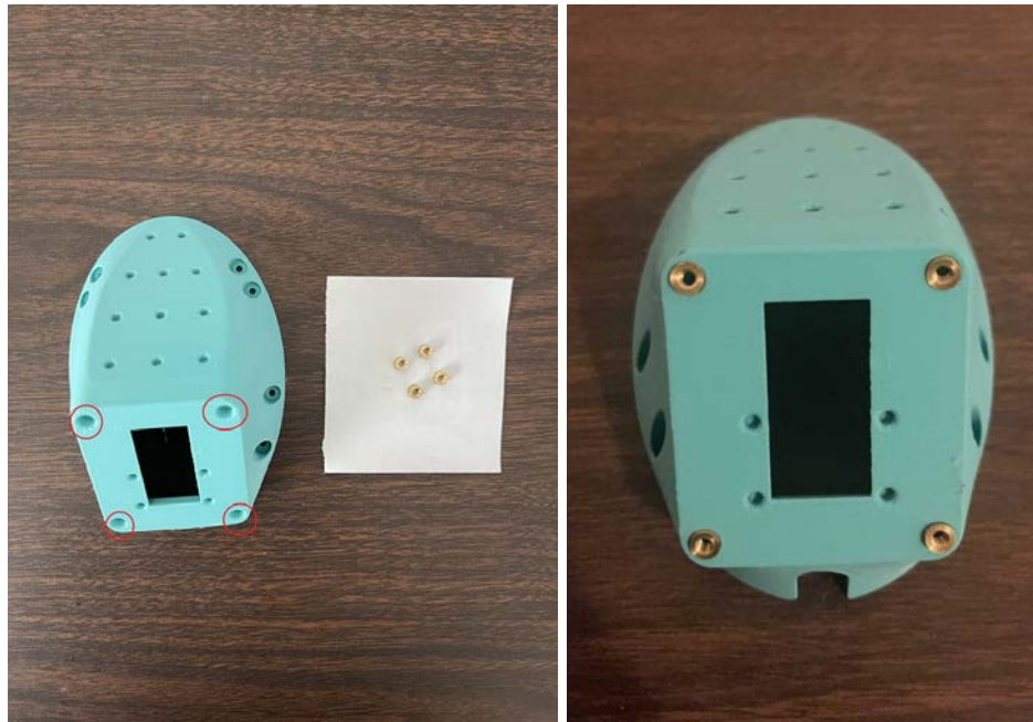
Figure 64: M3 heat-set insertion for part Bubble_Gripper_Body. Locations circled in red.
