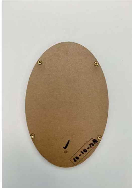
Figure 34: Marked tapped hole on acrylic window
