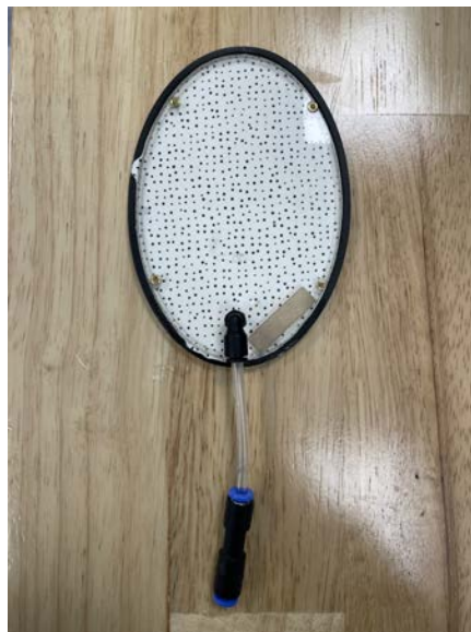
Figure 57: Completed assembly of bubble module
