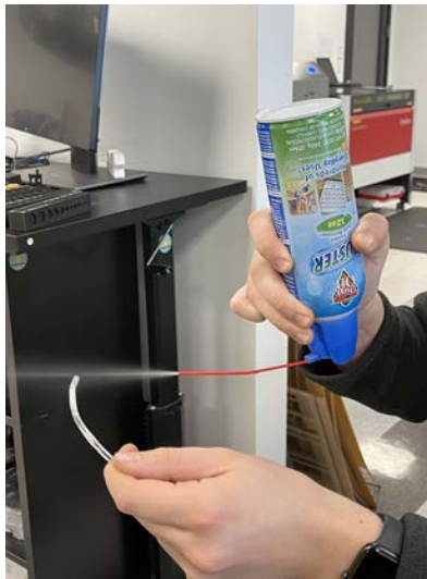
Figure 2: Compressed air duster is used to frost the tubing before connector insertion
