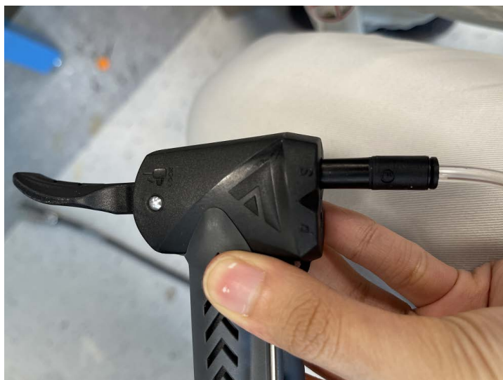
Figure 5: Connector-tubing assembly with sealed pump
