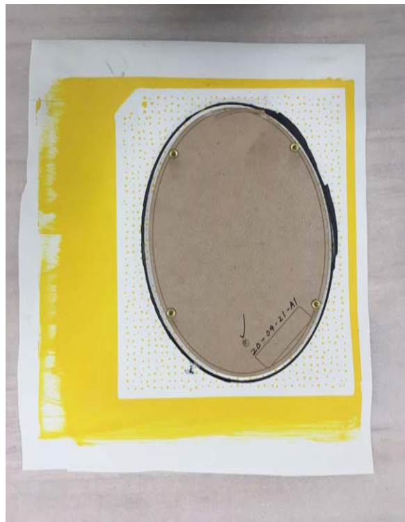
Figure 50: The latex cutting template is traced
