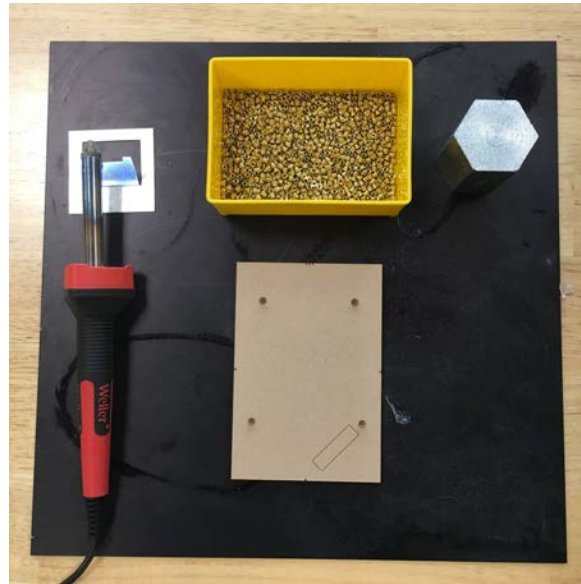
Figure 23: Tools and materials required to install heat-sets
