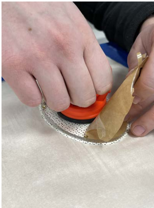
Figure 52: Apply suction cup to bubble module
