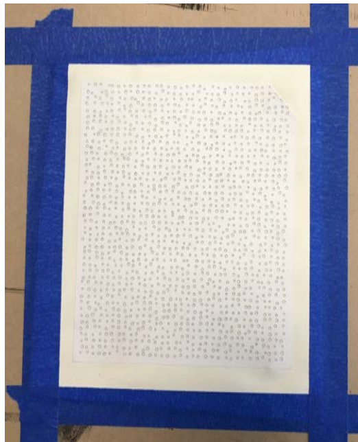
Figure 13: Stencil applied to latex after adhesive backing removed.
