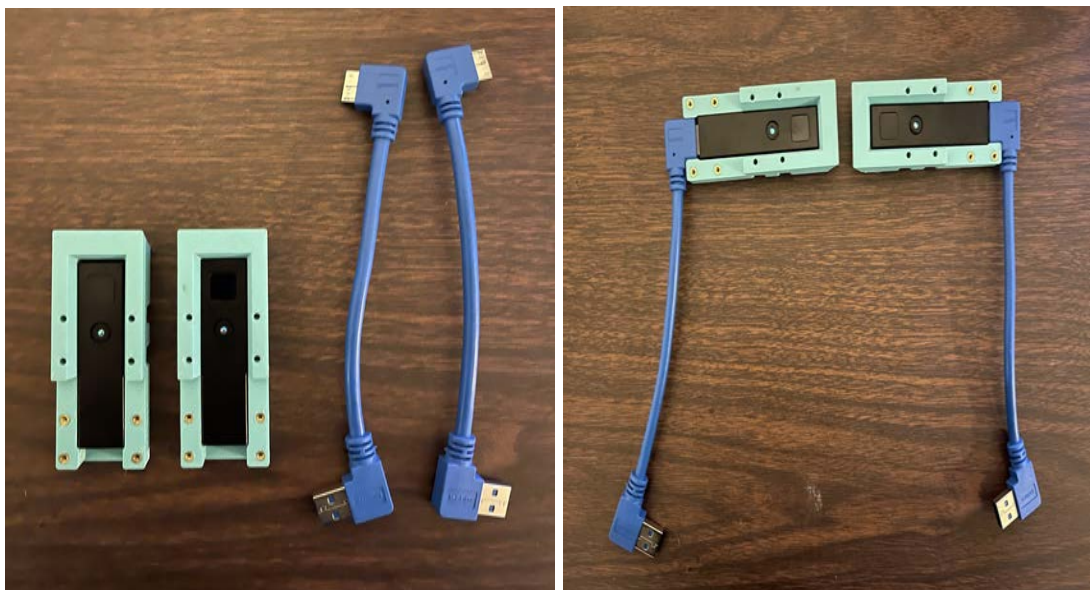
Figure 69: Right and Left USB cables inserted into Pico Flexxes
