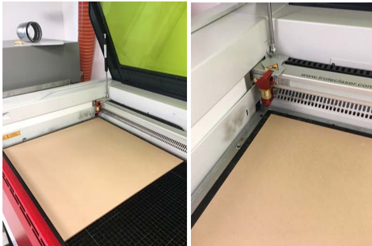
Figure 21: Alignment of acrylic into the laser cutter
