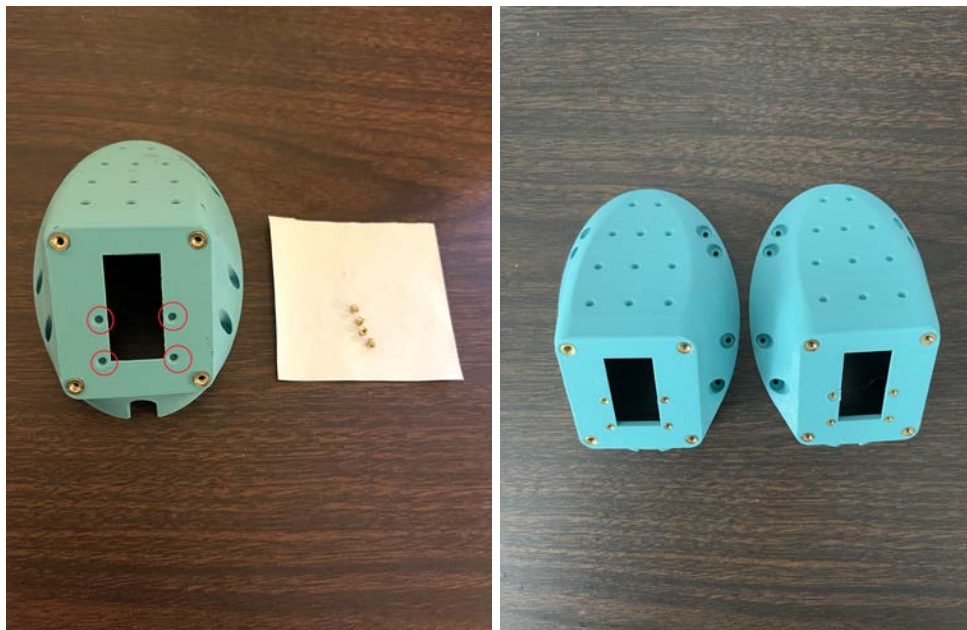
Figure 65: M2 heat-set insertion for part Bubble_Gripper_Body
