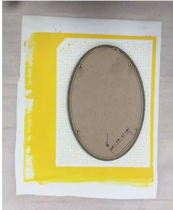
Figure 49: The latex cutting template placed around the adhered window
