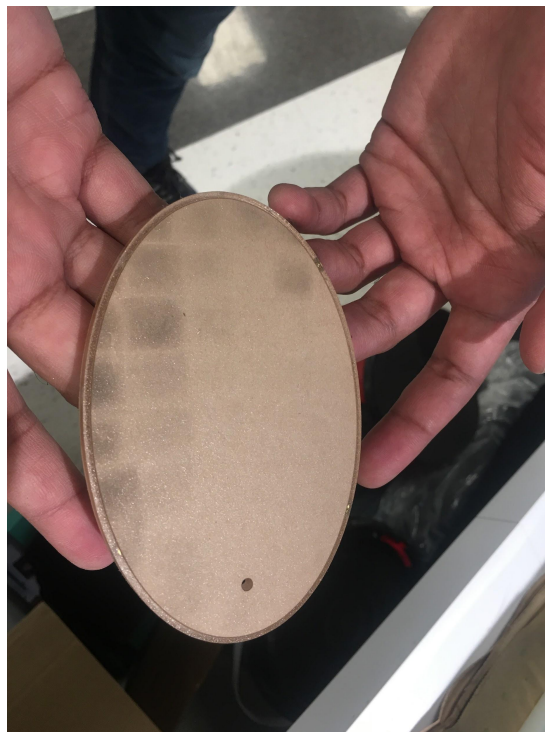
Figure 52: The surface of the acrylic is shiny and tacky after the repositionable adhesive spray.
