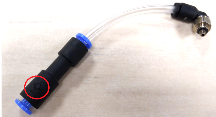
Figure 42: Completed bubble fitting-tubing assembly
