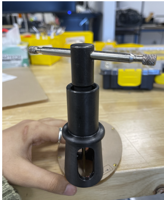
Figure 36: M3 tap is used to thread the air fitting hole
