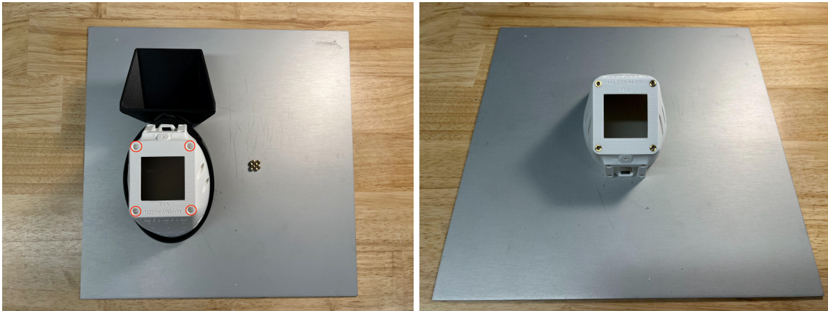
Figure 72: Left, the four locations for four M3 3.8 mm depth heat-set inserts are circled in red Right, the Bubble Gripper Body with the inserts installed.
