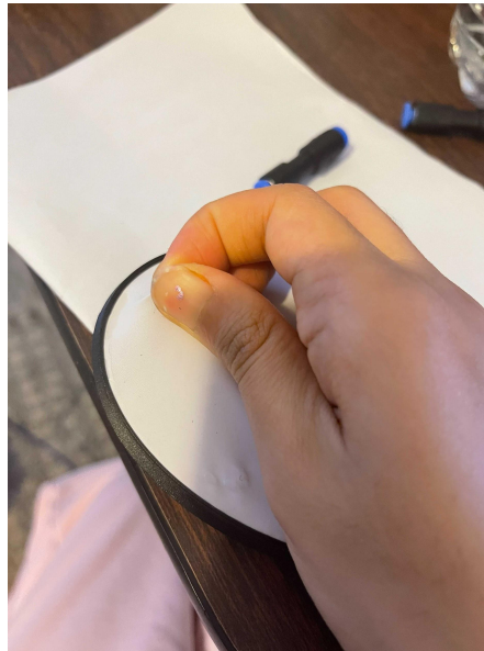
Figure 66: Pulling off latex that is stuck to the acrylic
