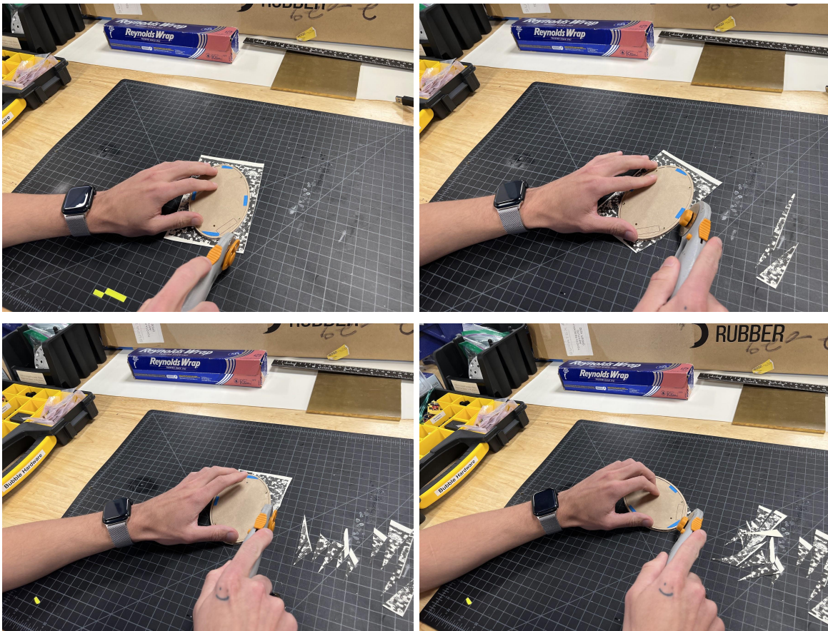
Figure 55: Using the rotary blade to trim the excess latex
