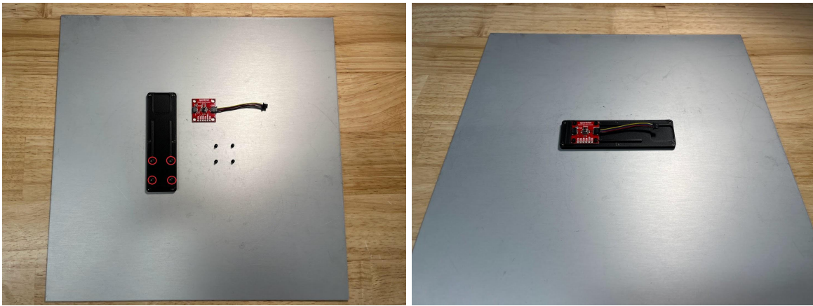
Figure 87: Locations and fasteners necessary to attach the pressure sensor board to Electronics Enclosure Bottom
