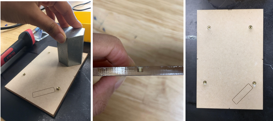
Figure 29: Insulated flat weight applied to the heat-set for flush insertion into pocket
