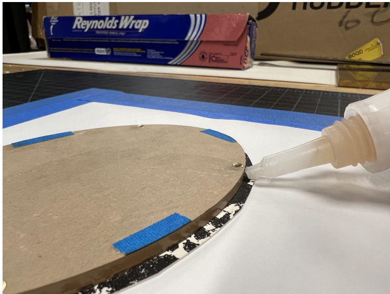
Figure 59: Glue is applied to the seam between the acrylic window edge and latex
