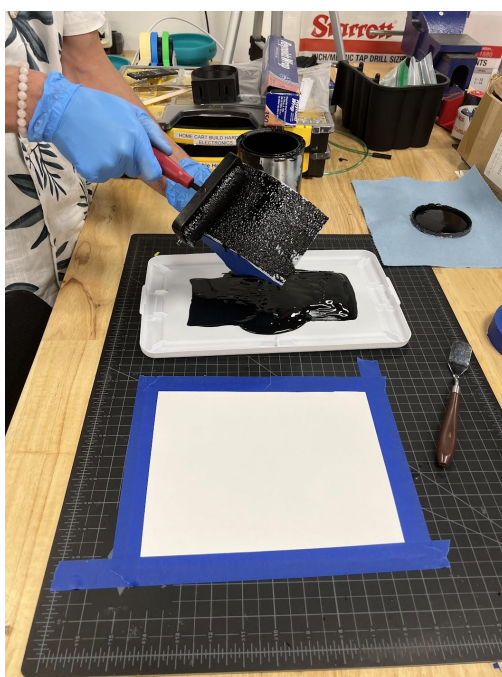
Figure 16: Using the brayer to apply ink to the Internal Pattern Stamp
