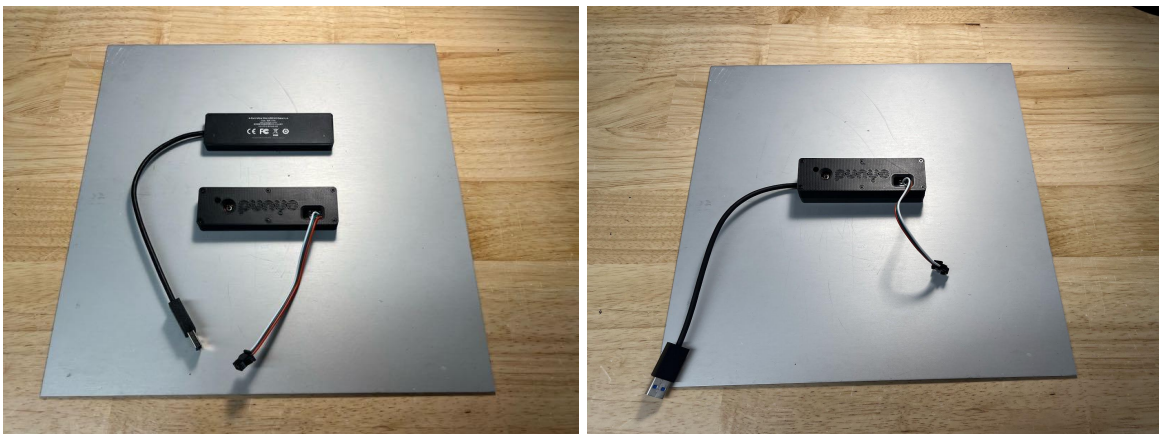
Figure 99: Orientation of the Pressure Sensing System and Anker USB hub before gluing together, and the combined unit
