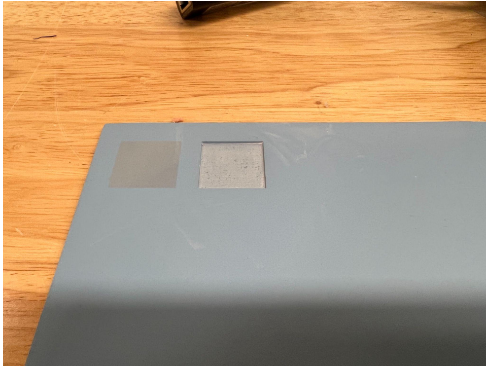
Figure 6: A 1 cm square with depth 1 mm etched into the rubber sheet
