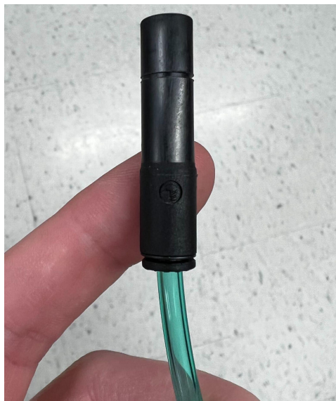
Figure 1: Tubing inserted into the push-to-connect end of fitting
