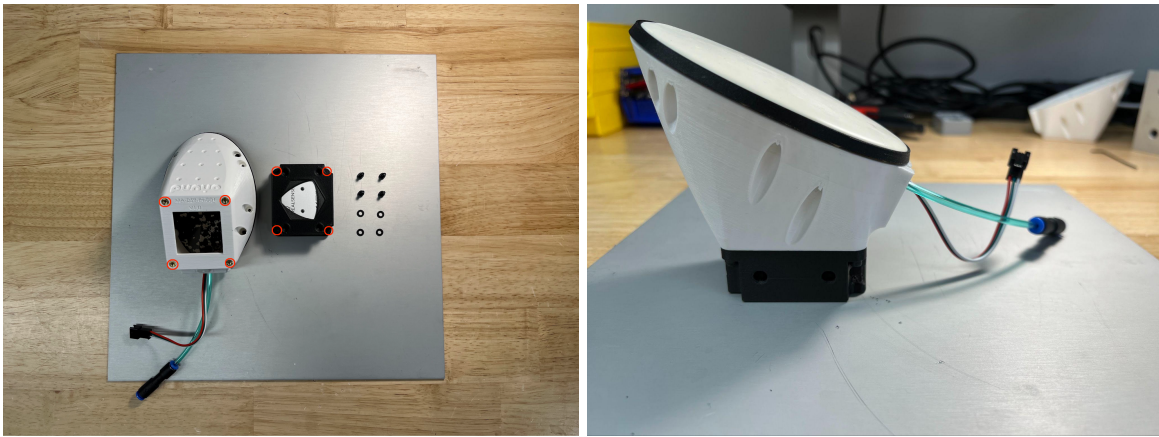
Figure 78: Locations and fasteners necessary to attach the Intel D405 Case to the Bubble Gripper Body
