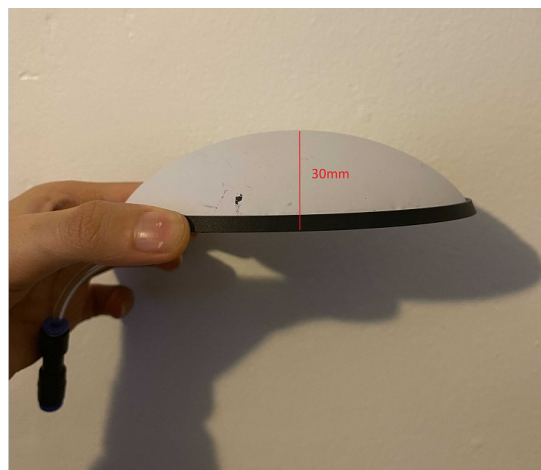
Figure 65: Inflated bubble module to a height of 30mm
