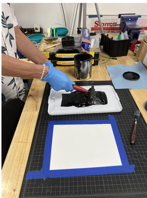
Figure 15: Applying ink to the rubber brayer
