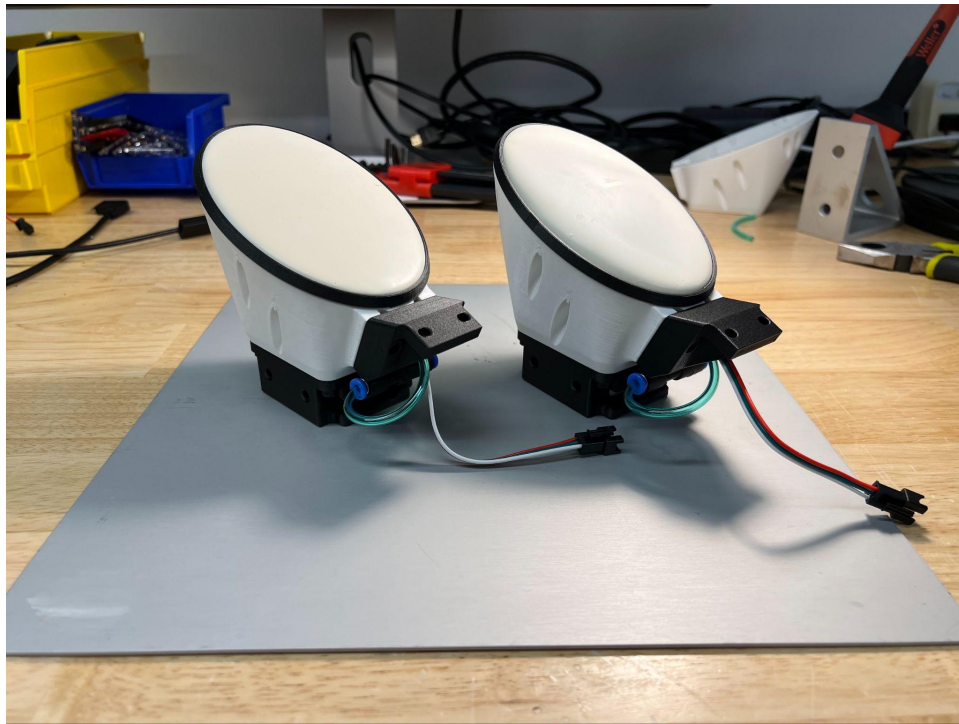
Figure 82: Two completed Punyo Soft-Bubble Gripper Fingers!
