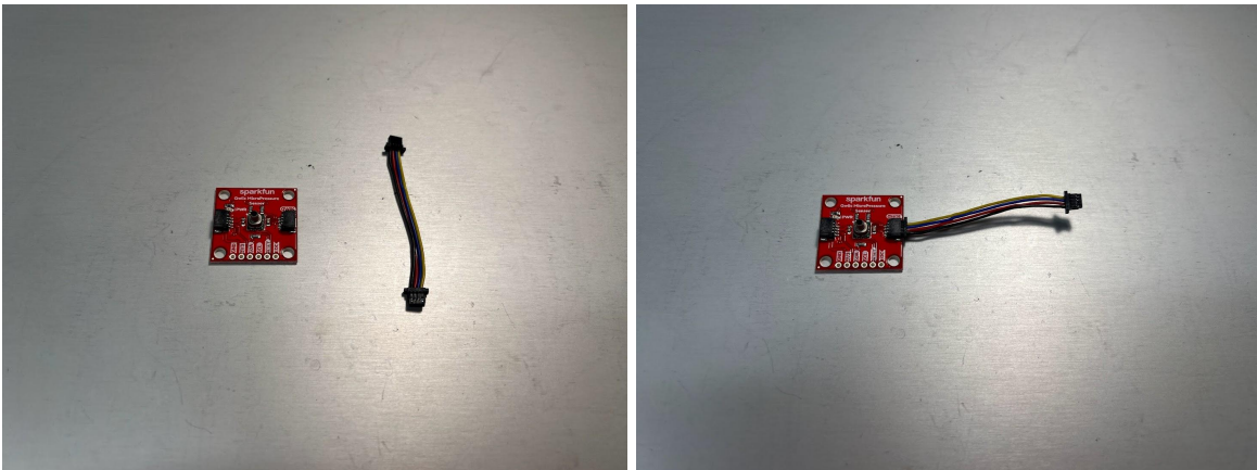
Figure 86: Sparkfun Qwiic MicroPressure Sensor with 50 mm Qwiic cable inserted
