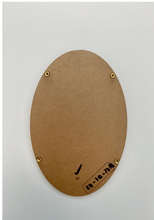
Figure 38: Marked tapped hole on acrylic window
