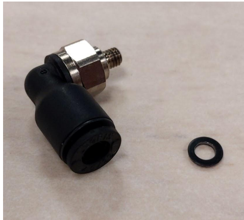
Figure 41: Swivel elbow push-to-connect fitting and O-ring
