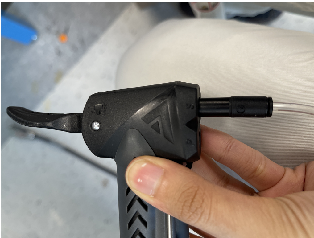
Figure 3: Connector-tubing assembly with sealed pump
