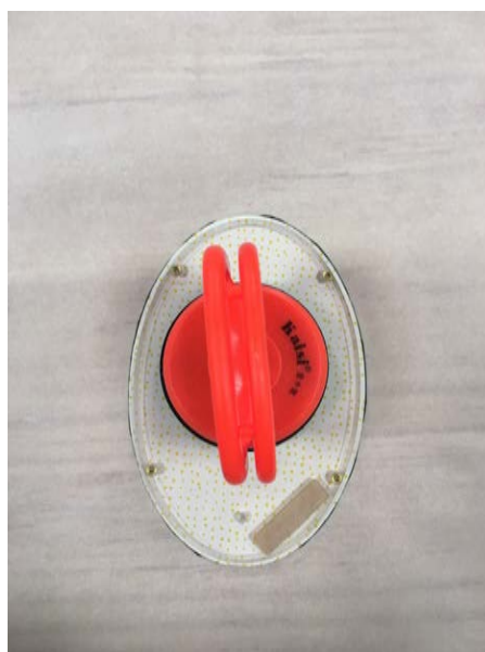
Figure 53: Final bubble module before sealing band application
