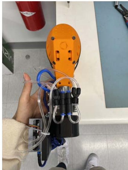
Figure 95a, 95b, 95c: Final Soft-Bubble gripper assembly with pressure sensing system
