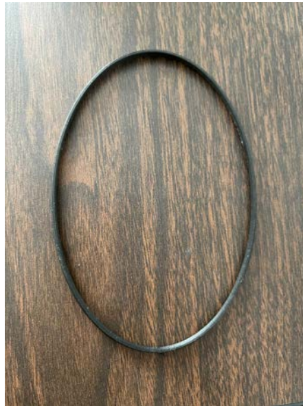
Figure 16: 3D printed 0.4 mm sealing band
