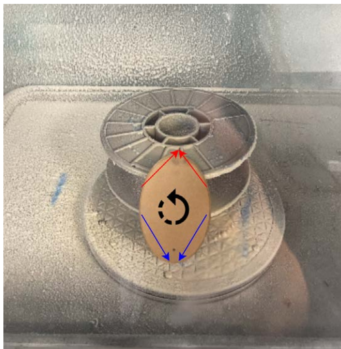
Figure 46: The adhesive is sprayed diagonally first in the red direction, then rotated as shown in black, and sprayed in the blue direction
