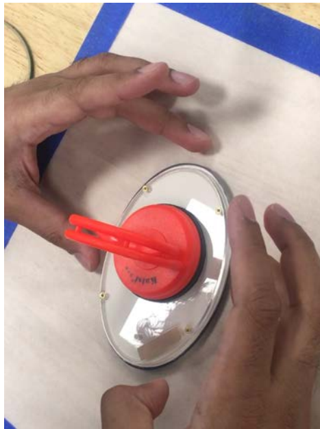
Figure 56: Alignment of bubble module over the sealing band
