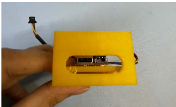
Figure 89: Microcontroller fixture is inserted with USB connector facing side opening.
