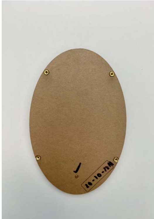
Figure 34: Marked tapped hole on acrylic window
