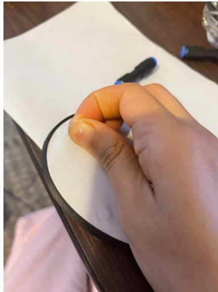
Figure 59: Pulling off latex that is stuck to the acrylic
