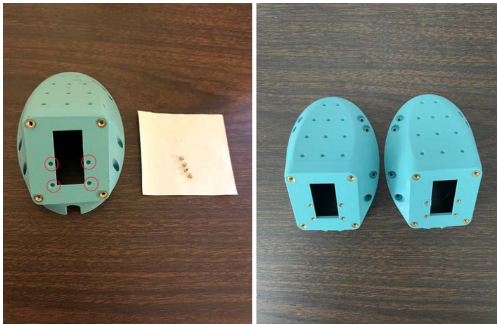
Figure 65: M2 heat-set insertion for part Bubble_Gripper_Body
