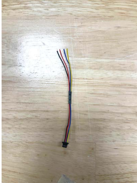
Figure 80: One connector end of the 100 mm Qwiic cable is cut off.
