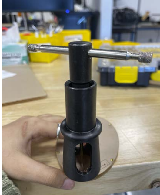
Figure 32: M3 thread is used to tap the air fitting hole
