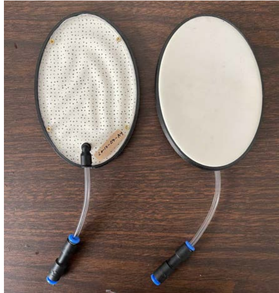
Figure 6: Fully assembled, deflated bubble modules, underside and top views
