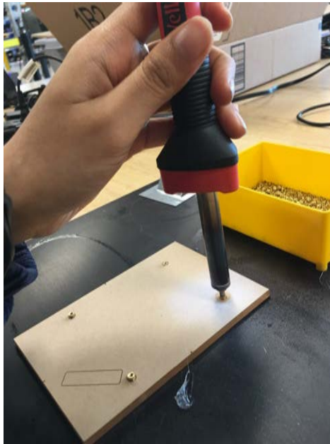
Figure 25: Sinking heat-sets into the acrylic window
