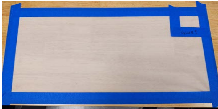
Figure 43: Parchment paper placed down and secured to the table
