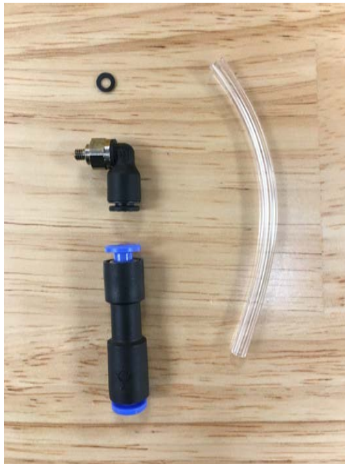
Figure 36: Materials for bubble fitting-tube assembly
