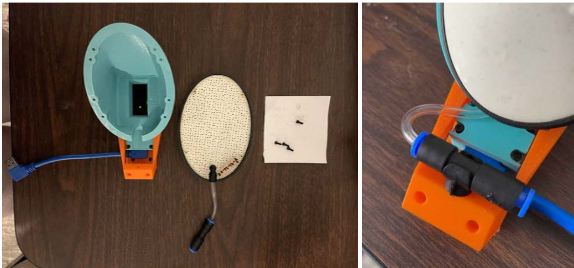
Figure 76: Push-to-connect fitting inserted into the clip
