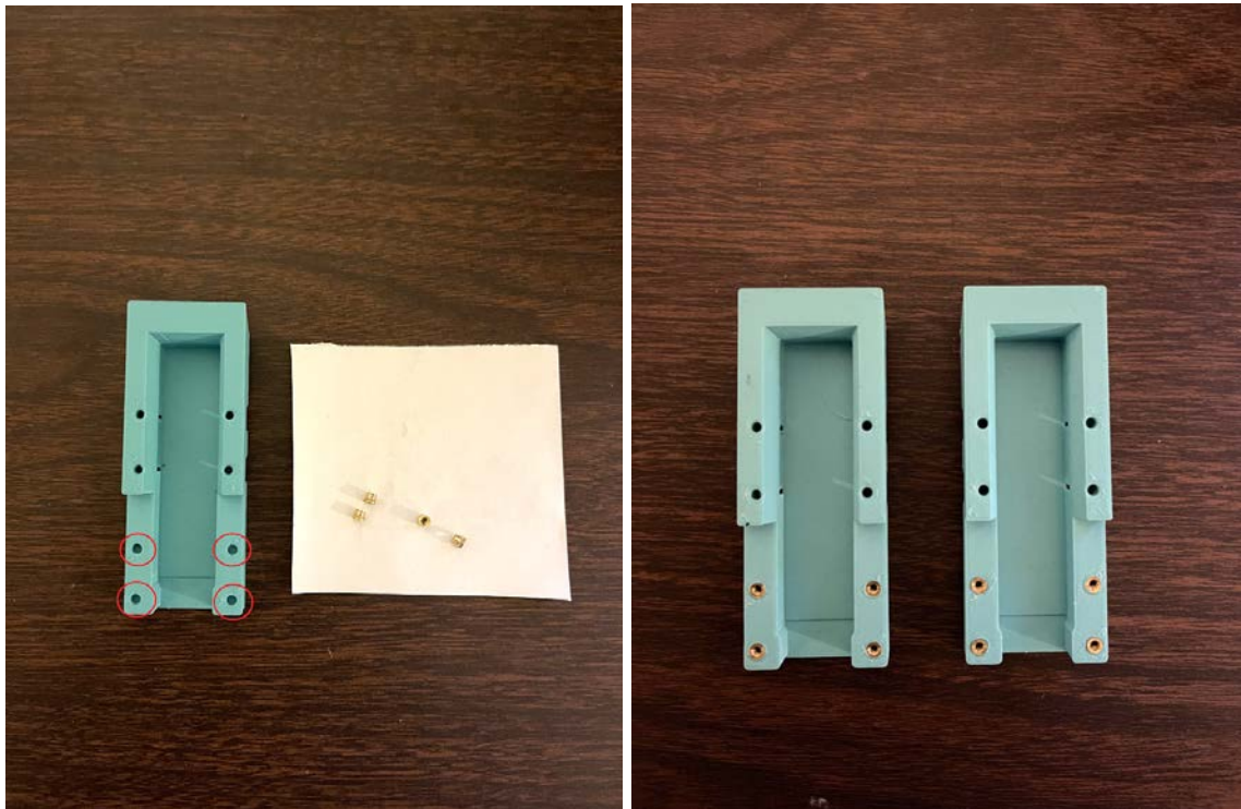
Figure 66: M2 heat-set insertion for part Pico_Case_Back
