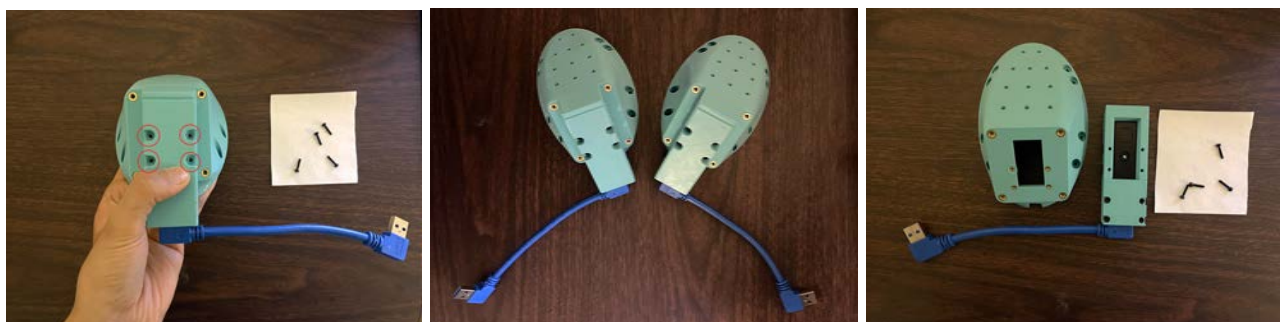
Figure 72: Mounting of part Pico_Case_Back onto Bubble_Gripper_Body
