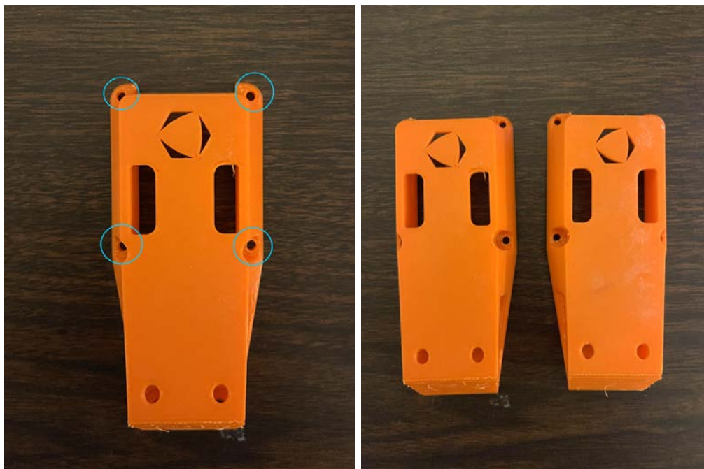
Figure 67: Removal of stray plastic in the holes of part Pico_Case_Front
