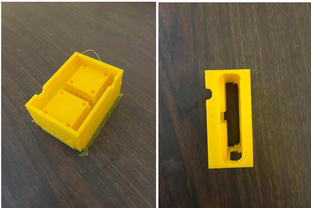
Figure 87: The support material is removed from the interior of the mount.
