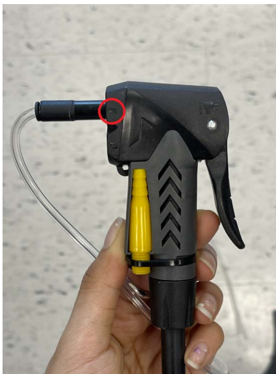
Figure 4: Connector-tubing assembly stuck into bike pump nozzle
