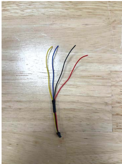
Figure 81: The four wires are peeled away from each other.
